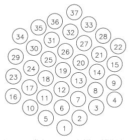
**Figure 1.** Arrangement of bolometers across the 850  $\mu$ m SCUBA detector array.
